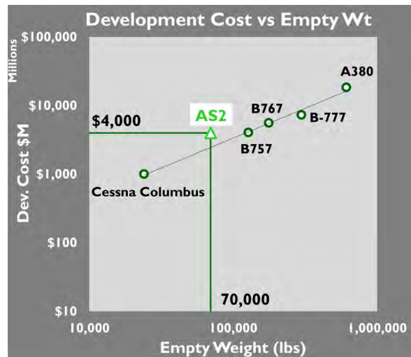
Figure 26 – Jet empty weight versus development costs, AS2 cost is 62% higher than that for subsonic models.
